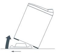
Fig.1 Tilt washer backwards to remove packer
